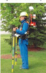
The Cath-Tech backpack is designed to dispense #32 gauge light survey wire. The backpack is equipped with a counter to measure the wire dispensed and can accommodate spools of wire up to 10 miles, 16 Km in length which minimizes down time for the survey crew.
