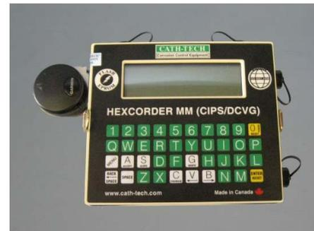
Figure 15 – Digital CIPS and DCVG meter
