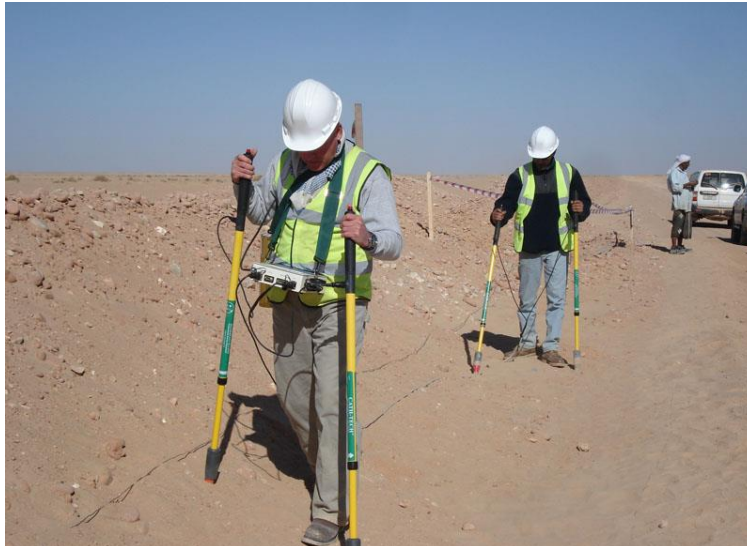
Figure 2 - Performing combined CIPS and DCVG survey with 4 poles
