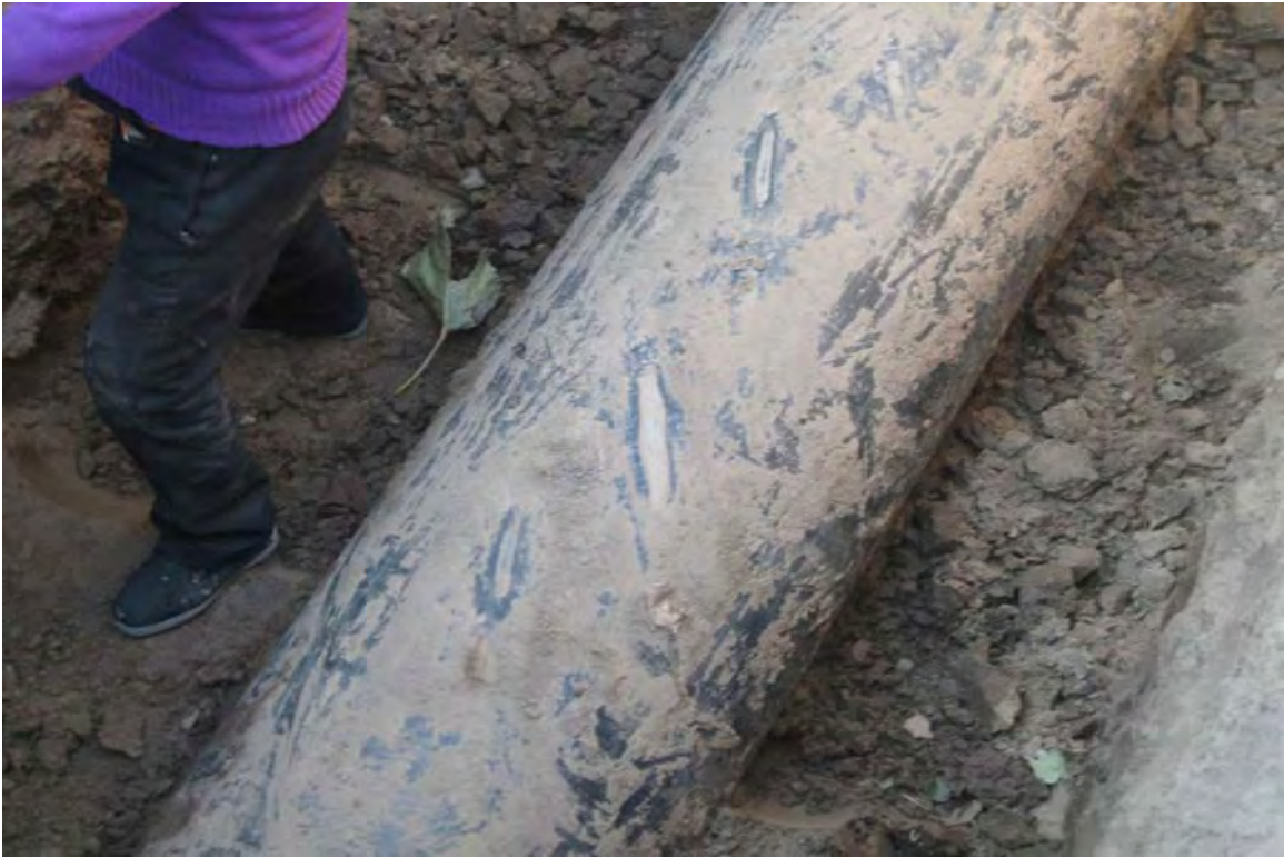
Figure15 Showing Backhoe Damage to Pipeline Coating
