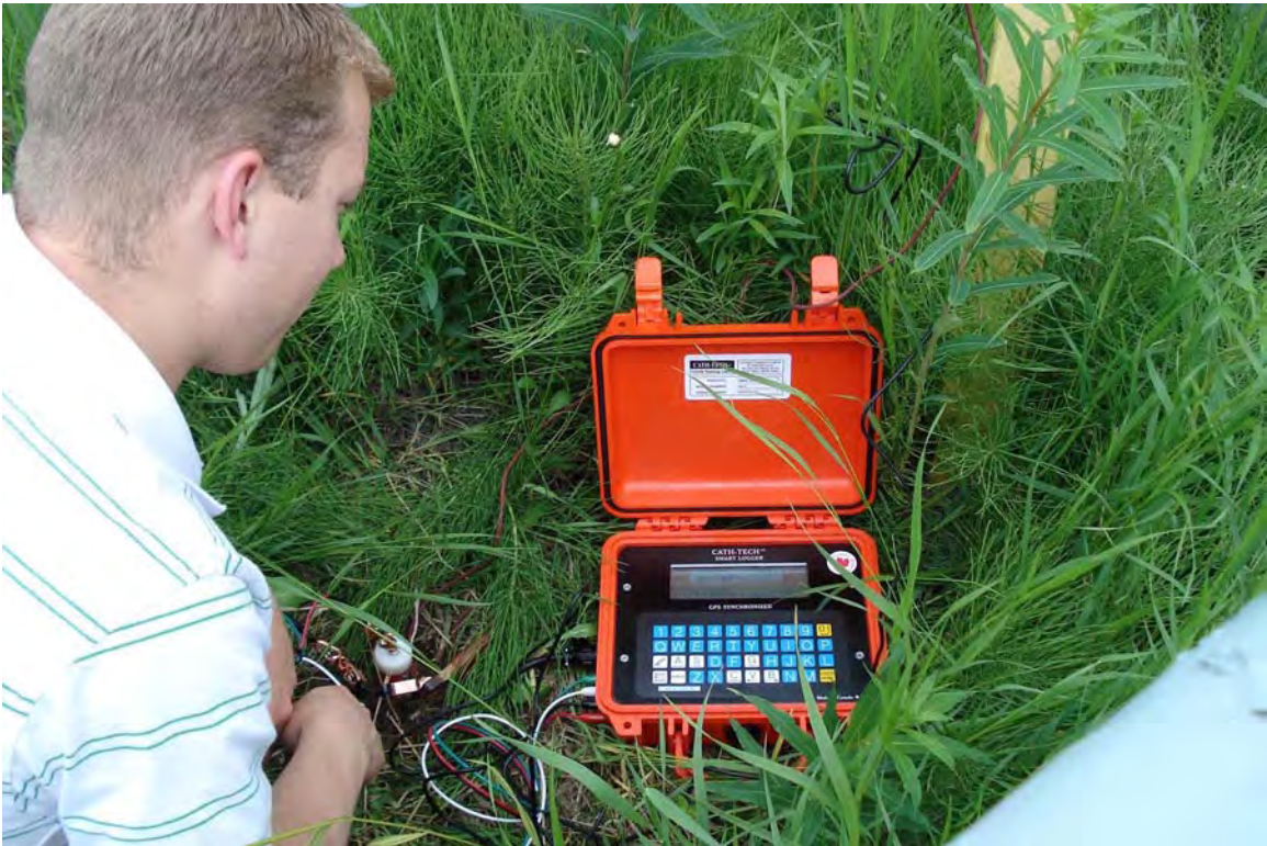
Figure16 Data logger With GPS Timing in Operation
