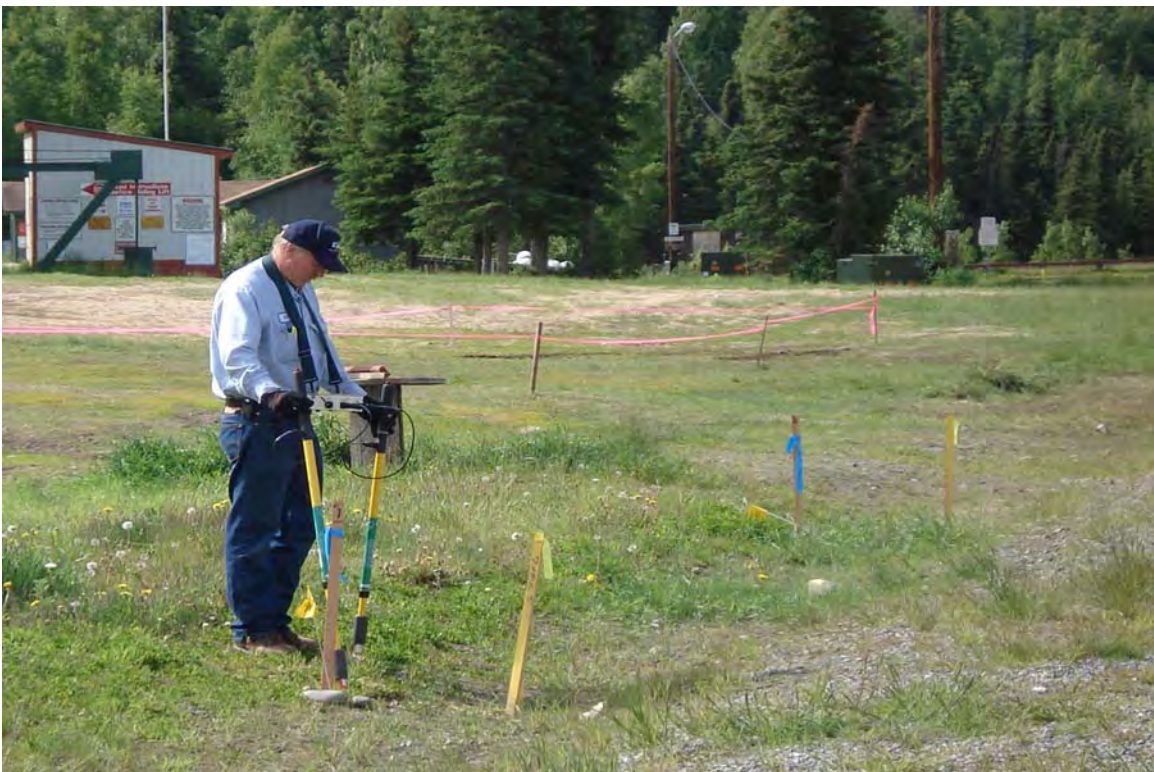
Figure 4 DCVG Surveyor with Stake-Outs of Defects
