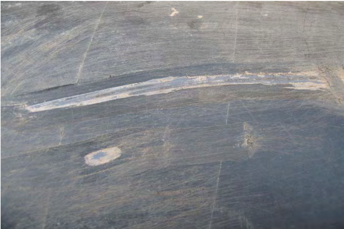
Figure 12 Coating Damage on a 20" Gas line
