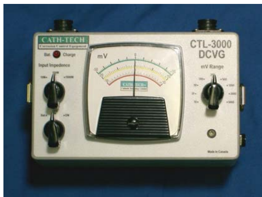
Figure 6 Analogue Direct Current Voltage Gradient Survey Instrument
