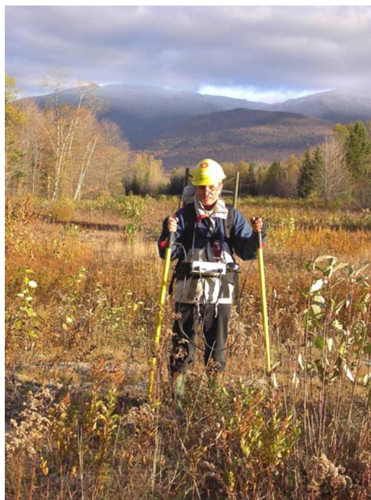
Figure 9 CIPS Surveyor with wire chainer and GPS system
