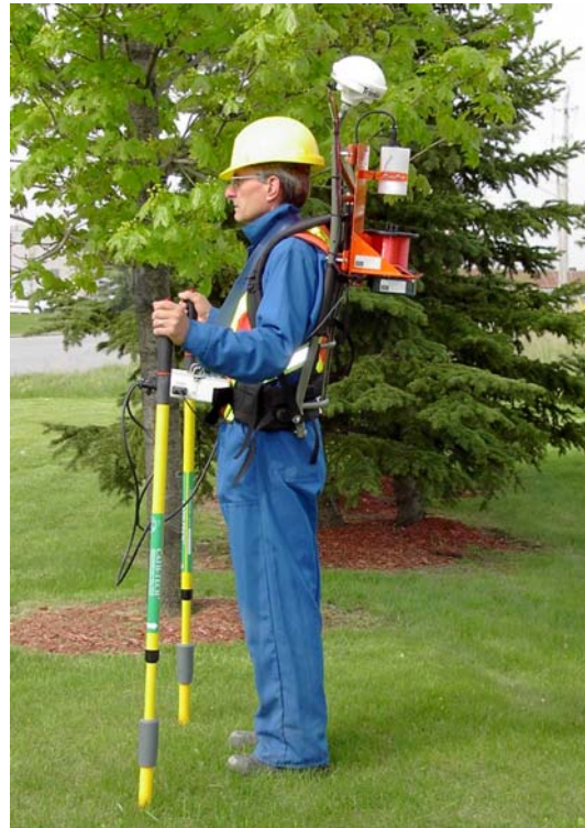
Figure 5 Close Interval Potential Surveyor with Sub-Metre GPS System
