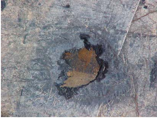
Figure 14 Defect located by CIPS + DCVG survey.
