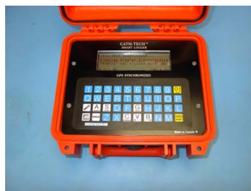
Figure 22 Stationary GPS Synchronized Data Logger. Cath-Tech Smart Logger Shown
