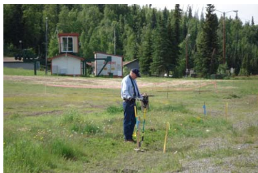
Figure 10: Staked out DCVG Indications
