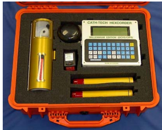
Figure 19 State of the Art CIPS + DCVG Survey Equipment. Cath-Tech Hexcorder Millennium Shown
