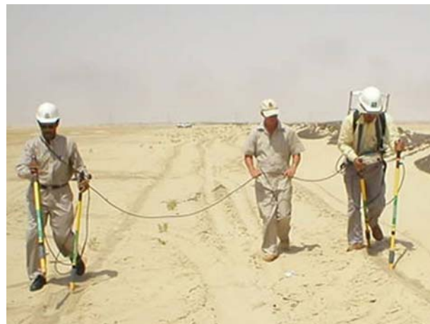
Figure 10 DCVG Measurement to Side of the Pipe
