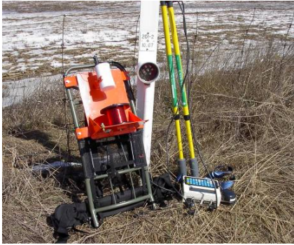
Fig. 3 - GPS Synchronized CIPS Survey Equipment, Cath-Tech Hexcorder
