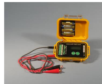
Fig. 2 - Small Stationary Logger, Cath-Tech MiniLogger
