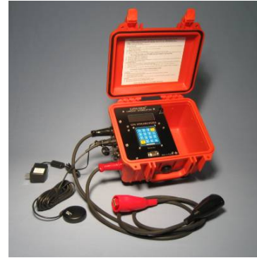
Fig. 4 - GPS Synchronized Current Interrupter, Cath-Tech CI-50
