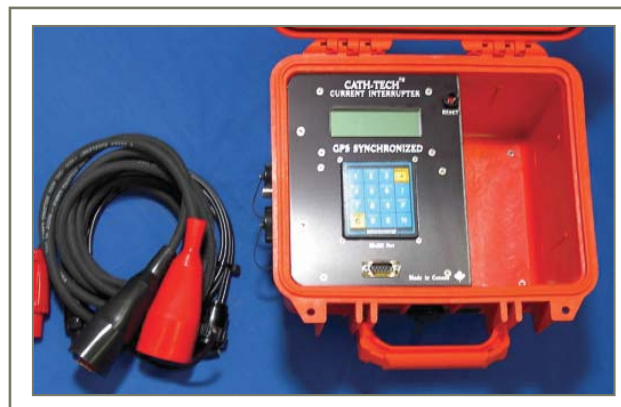
Figure 4. A modern GPS synchronised portable current interrupter.
