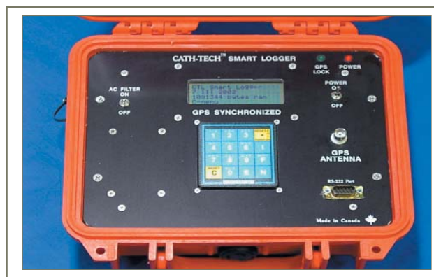
Figure 7. SmartLogger with GPS synchronisation logs the rectifier ON and instant OFF pipe-to-soil potential at each rectifier interruption.
