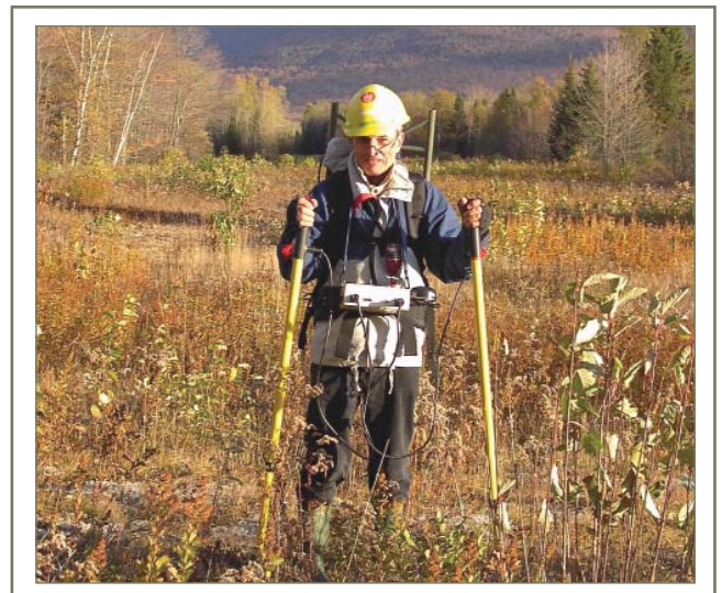
Figure 1. CIPS surveyor equipped with GPS data logger, trailing wire dispenser and half-cell poles.
