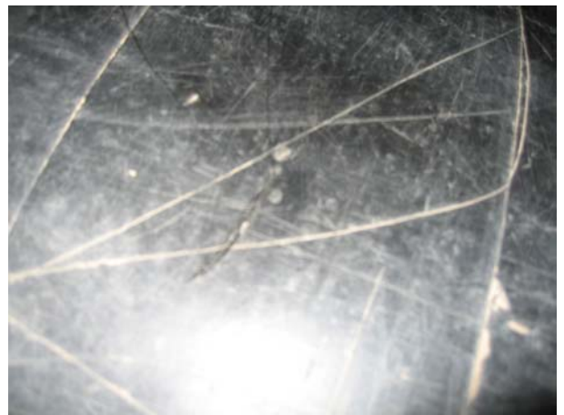
Photograph 5 Small Defect Detected by Combined CIPS and DCVG Survey
