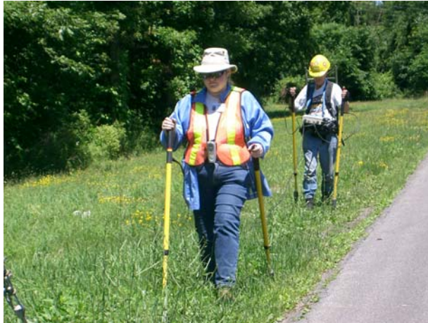
Photograph 4 Two Surveyors Performing a Combined CIPS and DCVG Survey
