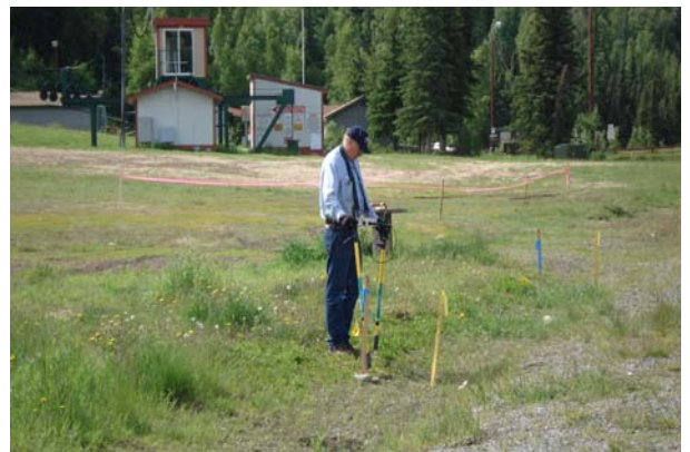
Photograph 2 Defect Stakeouts using Analogue DCVG Instrument
