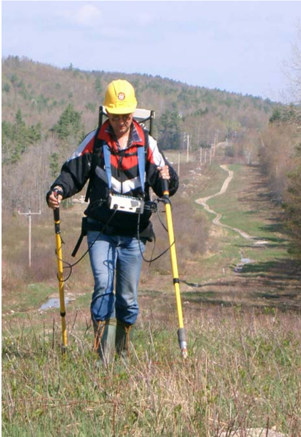
Photograph 1 a CIPS Surveyor at Work
