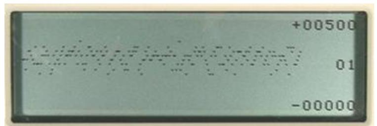
The first screen displays the first 100mS period following the start of the interruption cycle. This also, will normally be the start of the OFF period. Subsequent screens can be viewed, (100mS each), by pressing the arrow keys (V for left and B for right) to move back and forth through the waveform, the screen number is displayed on the right.
