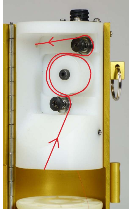
Figure 7 - Wire path through chainage counter
