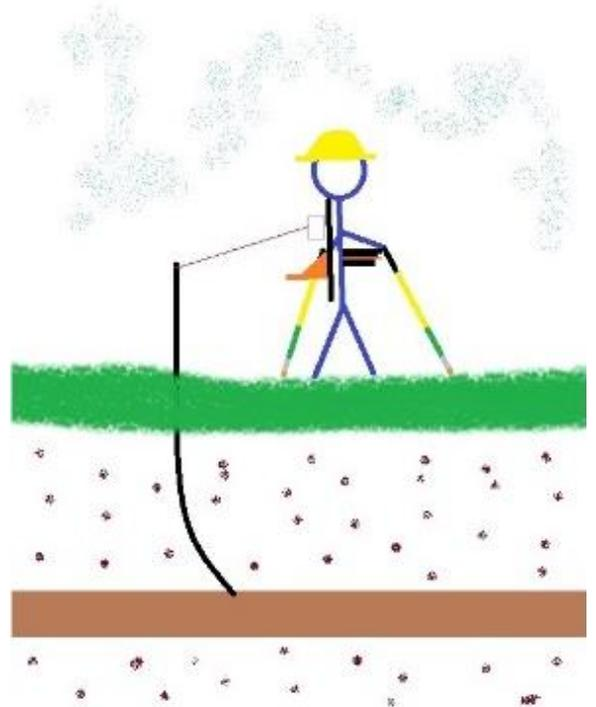
A close interval survey is best accomplished at a comfortable walking speed. Most surveyors prefer a 1 second cycle whereby the rectifier is turned OFF for 200 to 300 milliseconds every second. The one-second cycle will yield a stored reading approximately every two metres at a comfortable walking speed.
