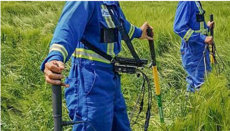
*Figure 8 - Two-man survey crew using Hexcorder Pro*
