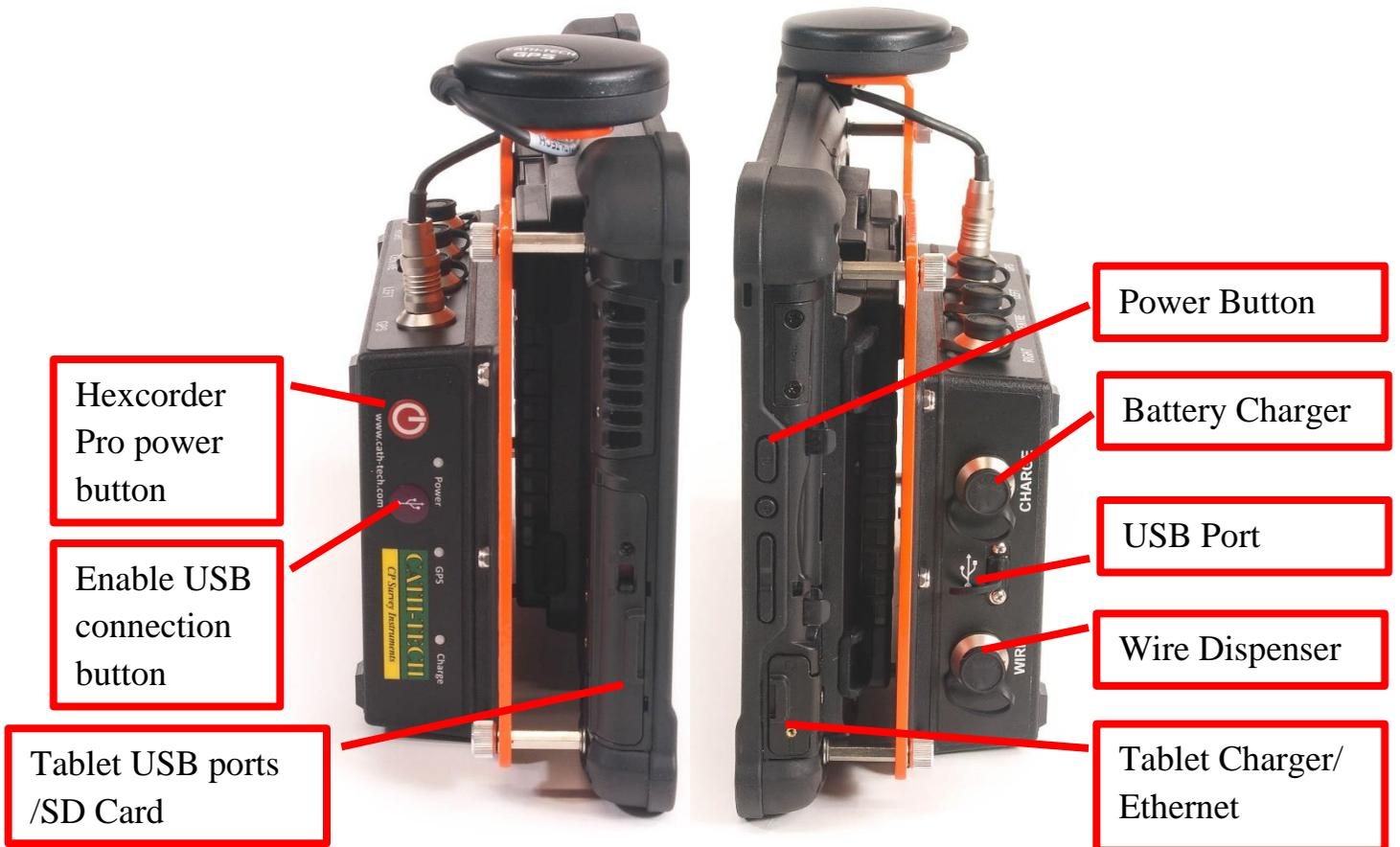
Figure 5 - Hexcorder Pro assembly - left view
