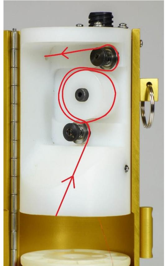
*Figure 7 - Wire path through chainage counter*
