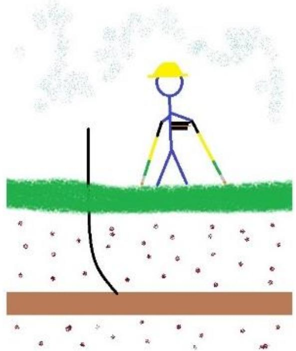
As a defect is approached a noticeable fluctuation is observed on the Hexcorder Pro at a rate similar to the interruption cycle. The amplitude of the fluctuation increases as the defect is approached. The swing of the values is directional, providing the probes are maintained in similar orientation parallel to the pipeline.
