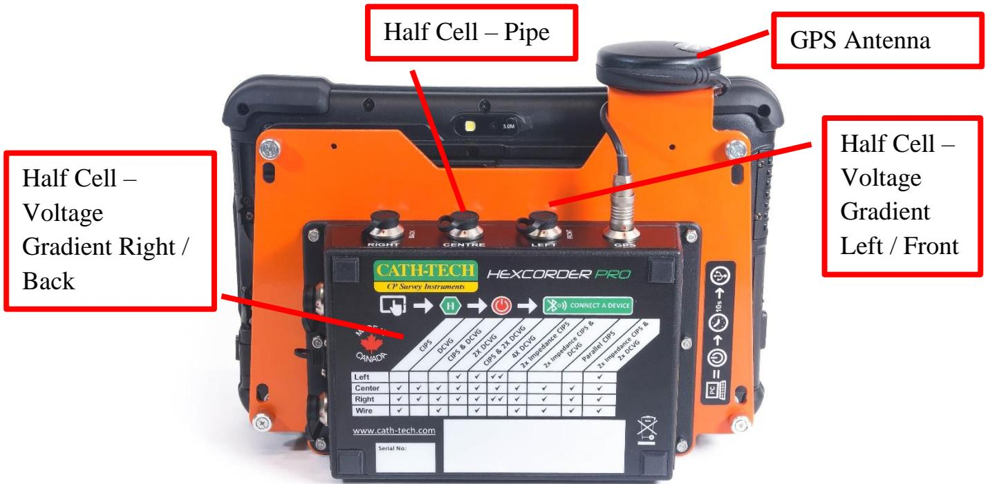
Figure 4 - Hexcorder Pro assembly - Bottom view
