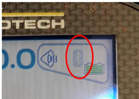
*Figure 27 - VM screen with Bluetooth disconnected*
