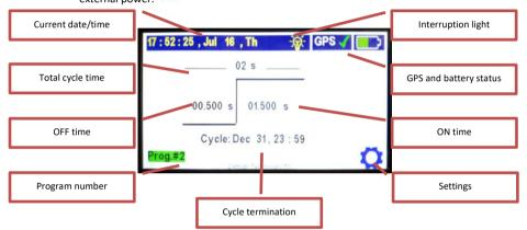
If the unit loses GPS lock, it will run off the internal clock until GPS is reacquired.
