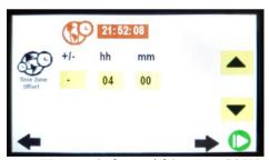
The user will see the current UTC time at the first row( if there is a valid GPS signal) and in the next row there are options to determine the offset to add to or subtract from the UTC time to adjust the unit's date and time according to the local time zone.
