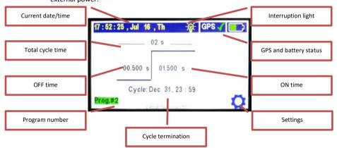
If the unit loses GPS lock, it will run off the internal clock until GPS is reacquired.
