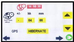
The user will see the current UTC time at the first row( if there is a valid GPS signal) and in the next row there are options to determine the offset to add to or subtract from the UTC time to adjust the unit's date and time according to the local time zone.
