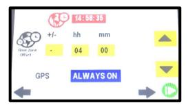
To save changes, the user must tap the **Forward** button. The inserted data will be saved and following message will be shown:
