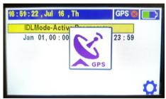
Upon successful GPS synchronization, the unit will go into operation and run whatever active programs it currently has stored. The amber INTERRUPT LED on the outside of the case will also begin to blink in time with the interruption cycle.
