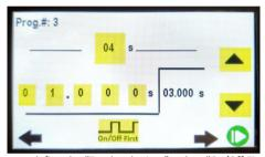
In this screen, the user must define the "Total cycle time", select "On/Off First" and define "OFF time". The "ON time" will be calculated according to the selected cycle time and OFF time.
