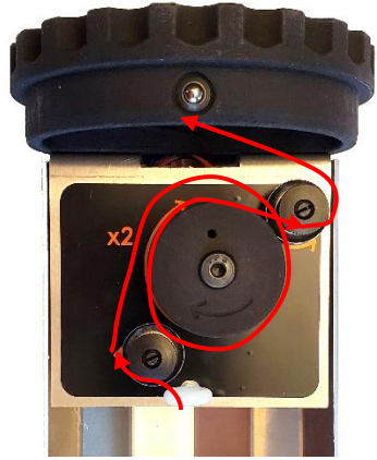
Figure 7 - Wire path through chainage counter
