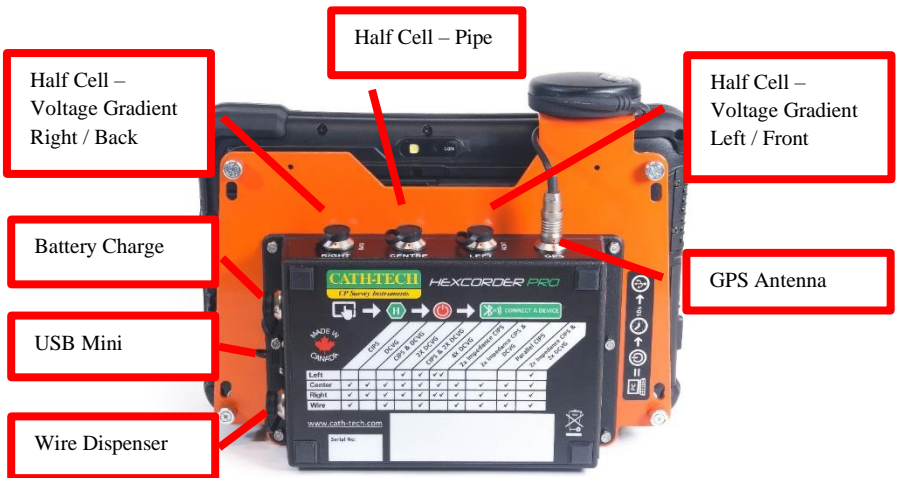
Figure 6 - Hexcorder Pro assembly - Bottom view
